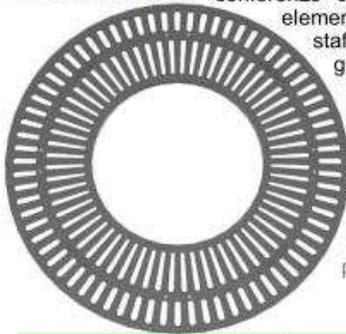
Cast-iron tree grate, PARIGI style, circular shaped, with slots located on 2 concentric circles, consisting of 4 modular elements assembled with cast-iron brackets and bolts inserted in the proper housings.
